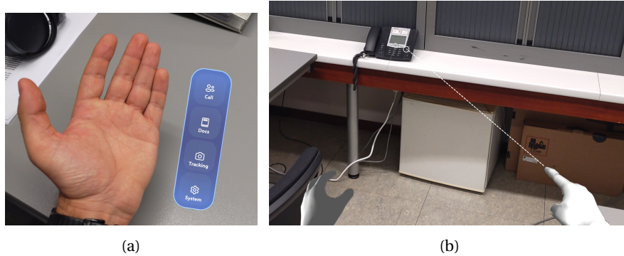
Figure 9.1: Illustrations of the prototype: (a) the hand menu and (b) a remote expert pointing to a phone.
