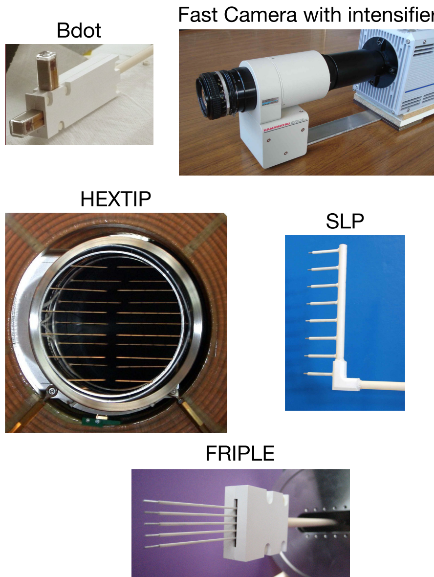
Figure 2.2 | Photographs of some of the main diagnostics used on TORPEX
