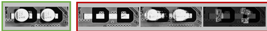
Fig. 8 (Color online) Zoomed area ( \approx X10 ) of a normal product image (left-green-framed 1st image) and an abnormal product image (right-red-framed image). One can see in the abnormal image that the input (2nd image) presents a pretty large defect (absence components), reconstructed with artefacts (3rd image) but still well patched (4th image).
