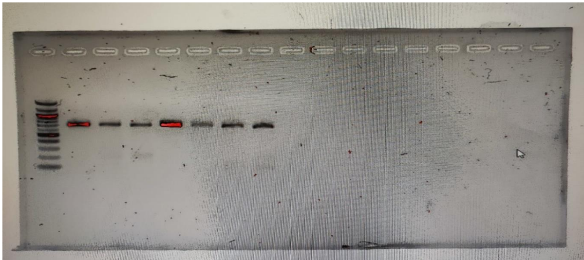
Picture showing an electrophoresis gel containing a ladder (for scale) and 7 successful PCR samples. The black bands show that there is DNA in our samples. So, we can send these samples to Sanger sequencing.
