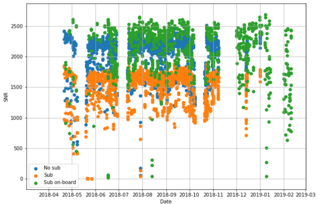
Figure 5.3: Mean SNR in the Sun region for on-board background subtraction (green), background subtraction (orange), and no background subtraction (blue).
