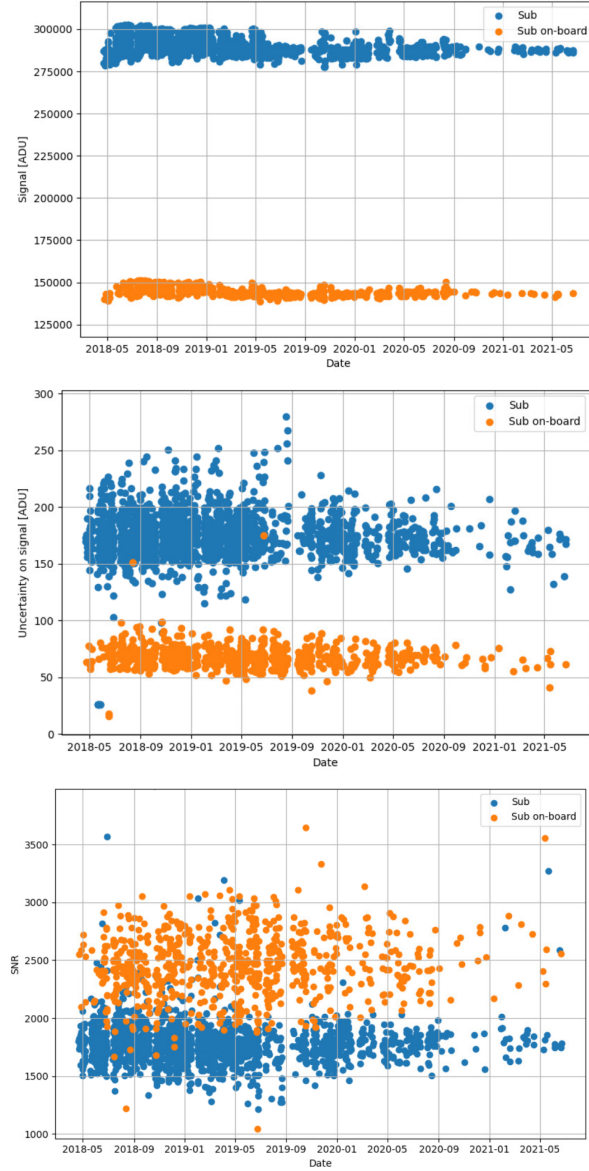
Figure 6.6: Mean signal (top), mean uncertainty on the signal(middle) and mean signal-to-noise ratio (bottom) in the S region for all datasets for diffraction order 168. Orange points are for datasets where the background is subtracted on-board TGO (before binning) while the blue points are for datasets with the background subtracted in the pipeline.
