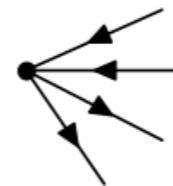
$$\mathbf{B}_1 = \begin{pmatrix} 1 & 1 & -1 & -1 & 0 & \dots & 0 \\ \times & \times & \times & \times & \times & \dots & \times \\ \vdots & \vdots & \vdots & \vdots & \vdots & \dots & \vdots \end{pmatrix}$$
