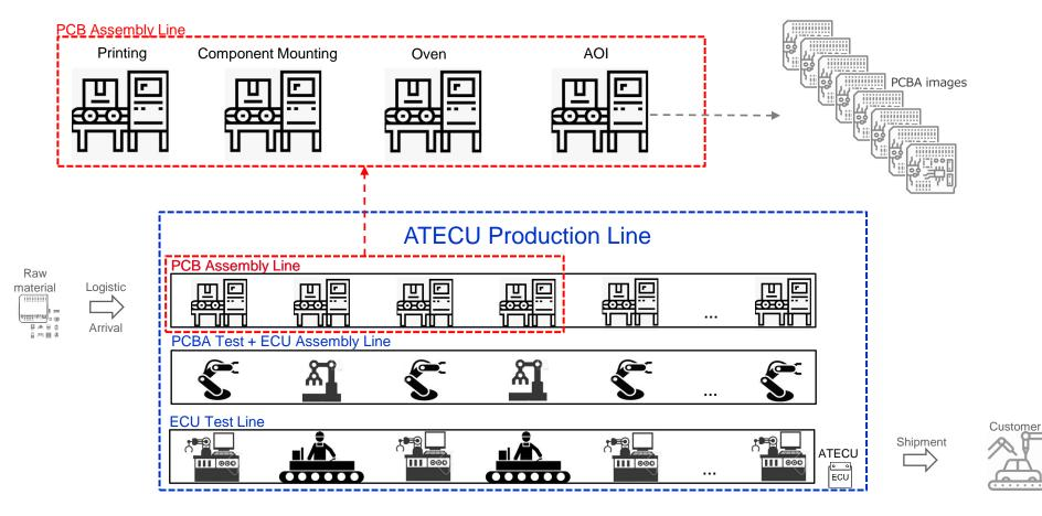
ATECU: Automatic Transmission Electronic Control Unit = finished product PCBA: Printed Circuit Board Assembly = intermediate product AOI: Automatic Optical Inspection = PCBA judgement process
