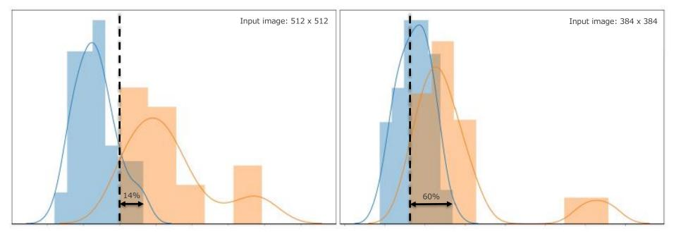
Anomaly scores for normal (blue) and abnormal (orange) images of the test dataset. The x-axis is the anomaly score of the test images and the y-axis corresponds to the score frequency.
