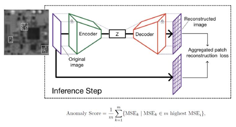
where m corresponds to the  $\alpha$ % of the patches with the highest anomaly score, and i is the patch index.
