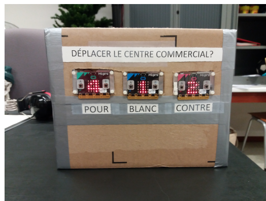
Figure 3. Vote counter displaying the aggregated results from the voting boxes developed by the children. The question asks children to express their opinions on the relocation of the mall.
