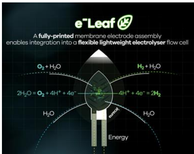
Figure V-50 – Schematic representation of the e - LEAF concept: a fully printed MEA in a flexible lightweight cell.
