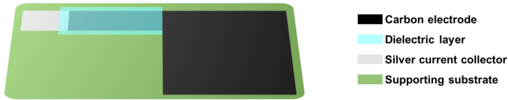
Figure V-7 – Illustrative representation of the complete screen-printed gas diffusion electrode containing a silver current collector, a dielectric layer in blue, and the carbon electrode. GDL design type B is represented.
