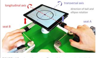
**FIGURE 1** Experimental apparatus. Two participants moved a virtual ball on a circular or elliptic target line. A universal joint underneath the tablet limited the motion space to motions around the longitudinal and the transversal axes. Each participant controlled one tablet axis with upward and downward movements of his index finger tip. Therefore, the task required the coordination of the individual actions.
