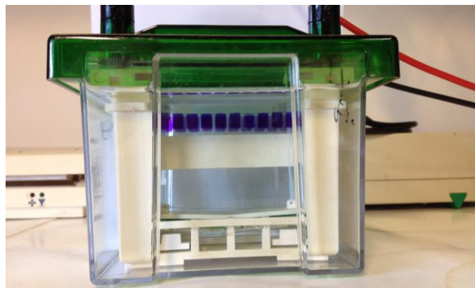
Figure 17: Mini-PROTEAN 3 system. Samples and standards are loaded in the wells made thanks to the comb. They appear in blue because dilutions were made thanks to the staining Laemmli. The picture was taken just before the electrophoresis migration of two hours.
