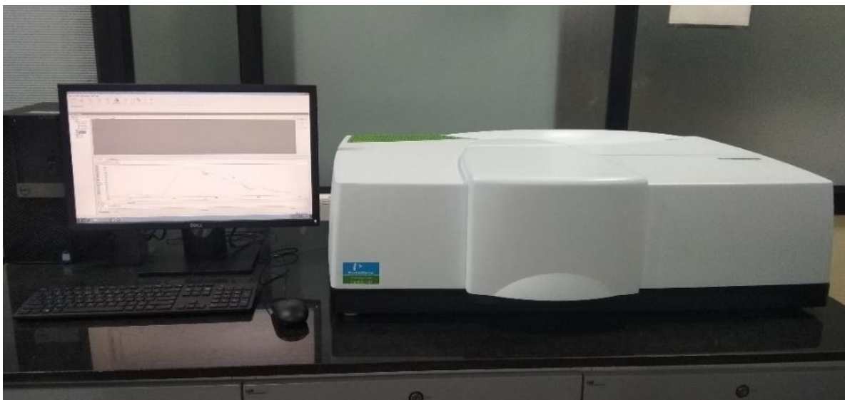
Figure A.5 LAMBDA 750 spectrophotometer.
