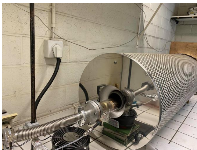
Figure 4.1 AP-CVD set-up used for the growth of MDs at the University of Namur.
