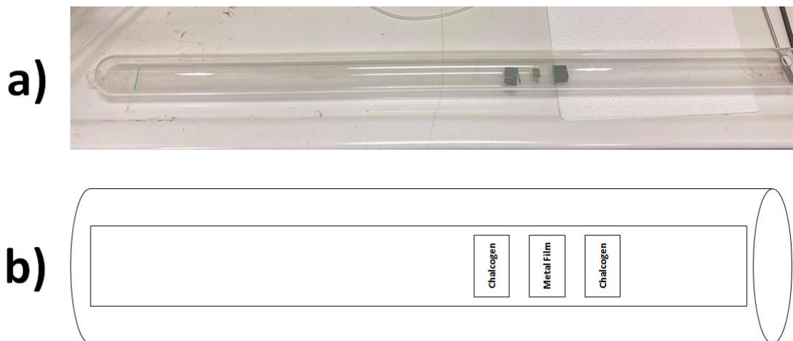
Figure 4.6 a) Quartz tube used during the MDs synthesis and b) schematic representation of the quartz tube.
