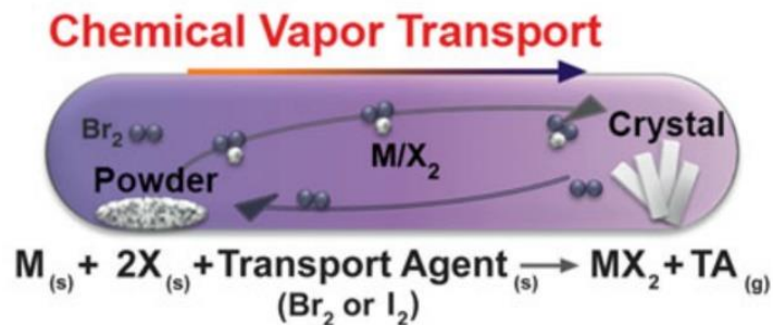
Figure 3.6 Schematic representation of Chemical Vapor Transport (CVT).
