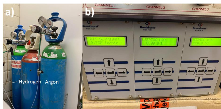
Figure 4.16 a) Bottoms of Argon (Ar) and Hydrogen (H 2 ) utilized during this thesis work and b) gas controllers.
