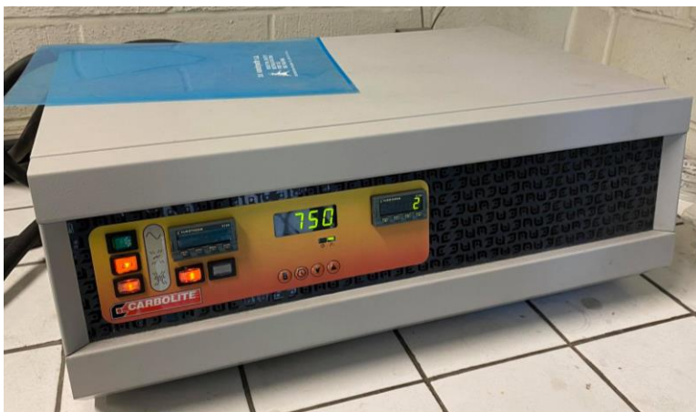
Figure 4.8 Temperature control system purchased from Carbolite.
