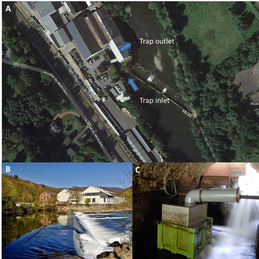
Figure 35: Trap location in Méry on the Rive Ourthe, (A) aerial vue, (B) side vue of the building beneath which the trap is located and (C) life-box at the end of the trap ( www.trekearth.com )
