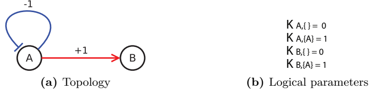
Figure 4.1: Example of a GRN with its topology (a) and its logical parameters (b). The delays associated with this GRN are \delta_{A,0^+}^{min} = 4 , \delta_{A,0^+}^{max} = 5 , \delta_{A,1^-}^{min} = 6 , \delta_{A,1^-}^{max} = 8 , \delta_{B,0^+}^{min} = 3 , \delta_{B,0^+}^{max} = 4 , \delta_{B,1^-}^{min} = 2 , \delta_{B,1^-}^{max} = 3 . Over each regulation, the sign and the threshold of the regulation are indicated.
