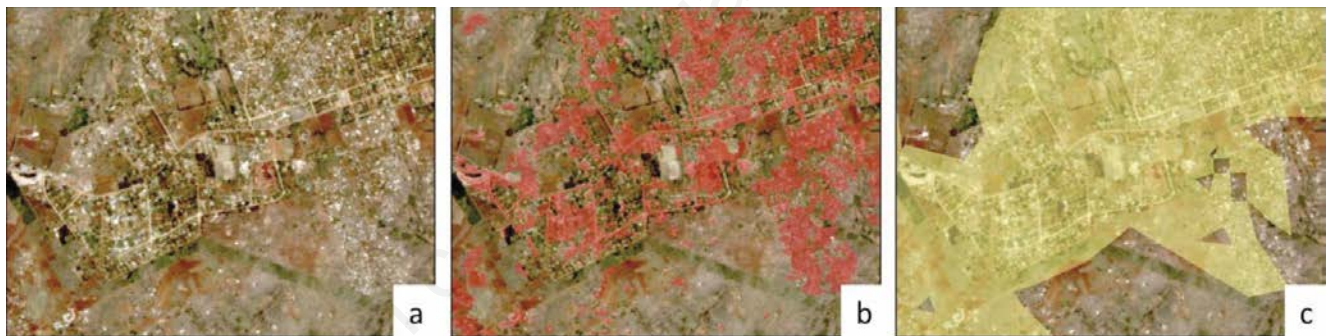
Figure 1. Example of settlement extraction. (a) RapidEye true colour composite (R:3, G:2, B:1), subset shows the city of Naamacha in Mozambique; (b) same image as (a) but with the outlines of the RapidEye derived settlements overlaid; (c) same image as (a) but with the outlines of the AfriPop settlements overlaid.
