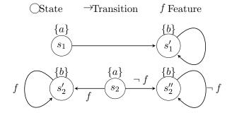
Figure 1: Two simulation-equivalent FTS.
